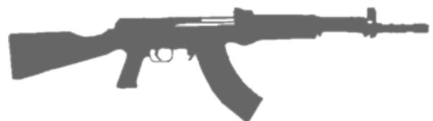
The Norinco Type 81 assault rifle entered into production and service in the early 1980s and is still being produced and offered for export sale. Its design and operating system incorporates elements of the Dragunov SVD, Simonov SKS, and AK-47 series rifles.
