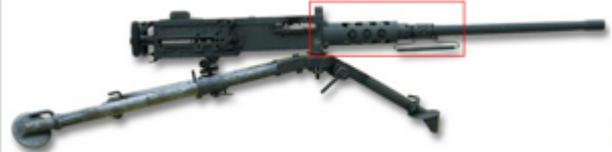
right view, Browning M2HB air-cooled machine gun on M3 tripod
