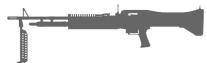
operation is unique, and drew on technical advances of the period, particularly the white "gas expansion and cutoff" principle also exploited by the M14 rifle. The M60's gas system was simpler than other gas systems and easier to clean.
