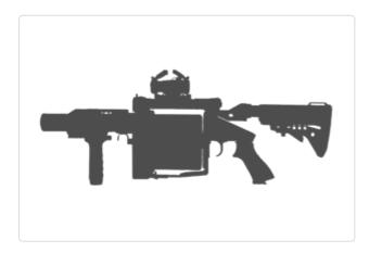
The Milkor (Milière Korporasie) MRGL (Multi-Range Grenade Launcher) is the fourth generation of six-shot launchers that was first introduced in the 1980s by the South African company and developed into a family with several variants. The MRGL fires with an effective range of 375 m to 800 m, depending on the ammunition used. The launcher is lightweight, semi-automatic, and shoulder-fired and can deliver its six rounds in less than three seconds.
