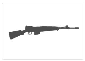
The MAS-49 is a French semi-automatic rifle that replaced various bolt action rifles as the French service rifle. The MAS-49 and MAS 49/56 use a direct gas impingement system with no gas piston. In this system gas is vented from a port on top of the barrel and piped directly into an open cylindrical hollow located in front and on top of the bolt carrier. The system has the advantage of not depositing gas fouling on the bolt itself, a separate part located underneath the bolt carrier. Many
