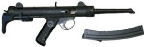
right view, Chilean copy of the Sterling submachine gun with external differences such as retractable wire stock and missing barrel shroud
