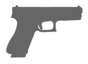
lack the holes in the barrel. The Glock 17MB is a version with ambidextrous magazine catch. Glock pistols are designed with three independent safety mechanisms to prevent accidental discharge. The system, designated "Safe Action" by Glock, consists of an external integrated trigger safety and two automatic internal safeties: a firing pin safety and a drop safety. The external safety is a small inner lever contained in the trigger.
