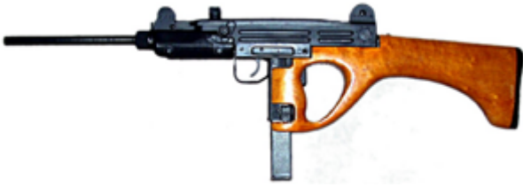
left view, , sporter model single action, semi-automatic
