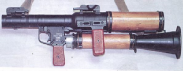
Version for airborne troops, disassembled for transportation / airdrop
