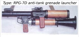
Version for airborne troops, disassembled for transportation / airdrop
